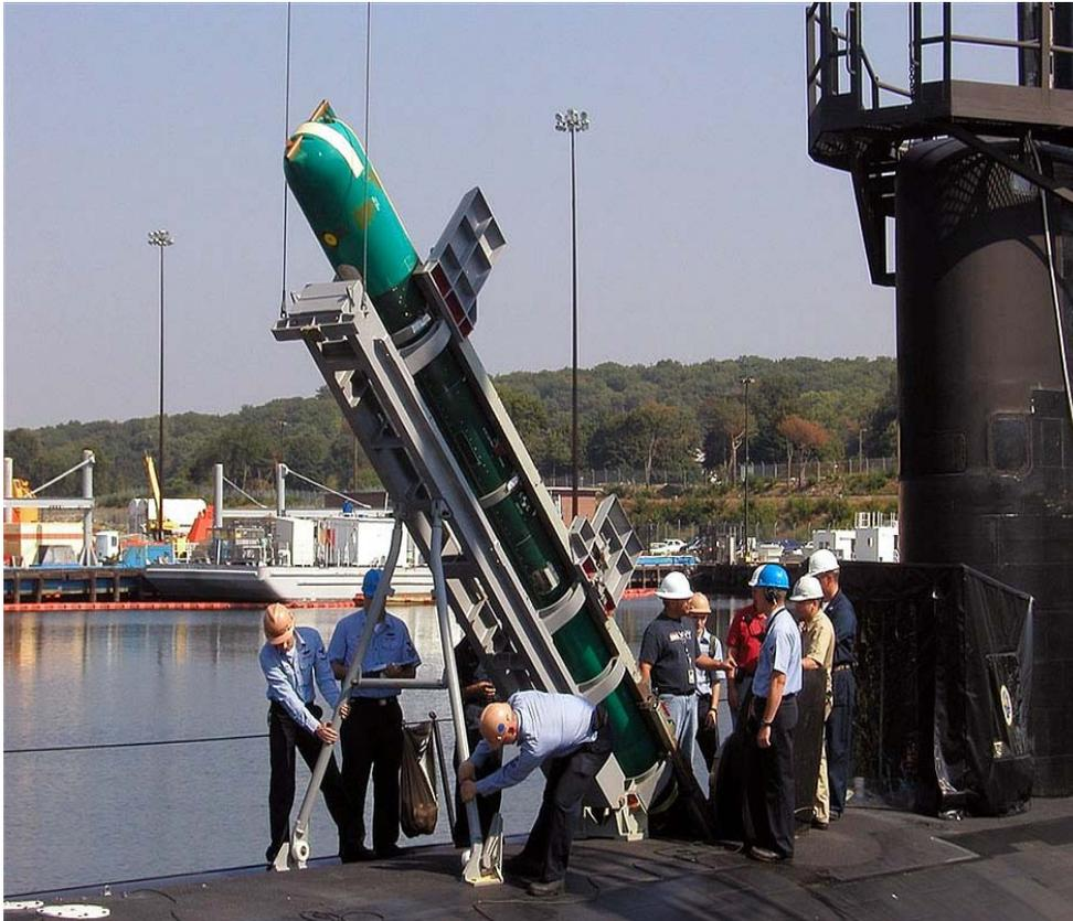
Boeing's AN/BLQ-11 has demonstrated the first ever 21' Unmanned Underwater Vehicle (UUV) autonomous launch and recovery operation from a submarine. Here, the vehicle and all its ship-board equipment is loaded into its host submarine the same way torpedoes are loaded. AN/BLQ-11 is designed to
