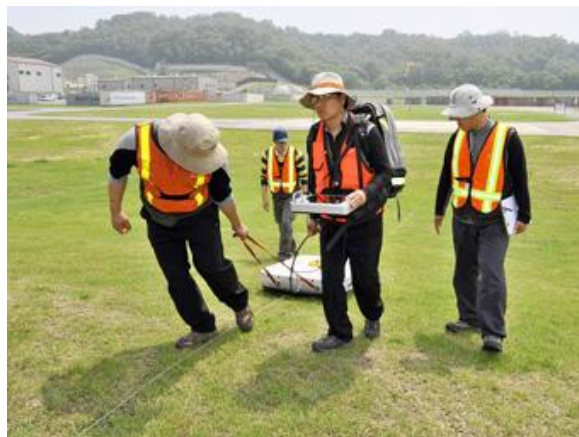
South Korean technicians conduct a ground-penetrating radar survey at Camp Carroll, a U.S. base in Waegwan, South Korea, to search for drums of Agent Orange possibly buried there.
